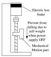
Note: The brake built in the servo motor is a fixed special brake without excitation. It can not be used for dynamic braking. Please use it only when the servo motor is in a stop state.
