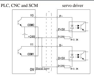
When the upper device adopts collector open circuit output, use this connection method, please pay attention to suspending P+ 5V and D+ 5V.
