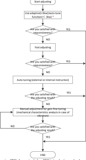
Note: \* marked as version 3730, the version before 3730 is in adaptive mode when out of factory.
