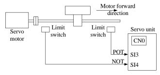
Rotary applications such as round tables and conveyors do not need the function of overrun prevention. At this time, there is no need to connect the overrun prevention with input signals.
