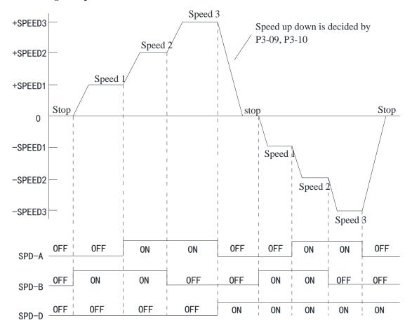
**5.4.3** Speed control (pulse frequency command)
