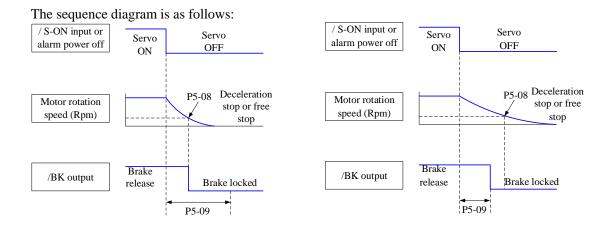
Since the brake of the servo motor is designed for position holding, it must be enabled at the right time when the motor stops. While observing the action of the machine, adjust the user parameters.
