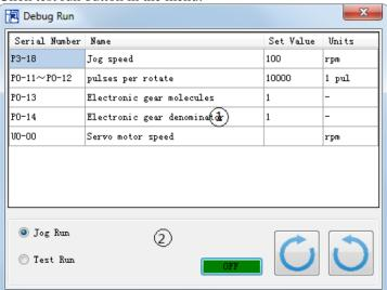
Jog speed P3-18: the motor speed in jog mode.
