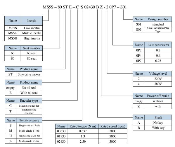
Note: At present, only the combination of CS, CM, TL and T is selected for the type of encoder.
