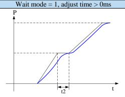
After the drive output 1-segment position command, it will not wait for the completion of motor positioning, but pass the adjust time, and then start the next position command. T2 is adjust time. Refer to parameter P4-11.
