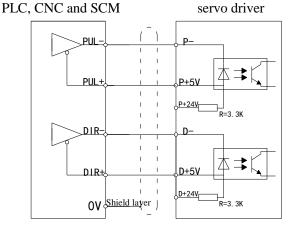
When the upper device uses 5V differential signal output, the graphic connection method adopted, please pay attention to suspending P+ 24V and D+24V.
