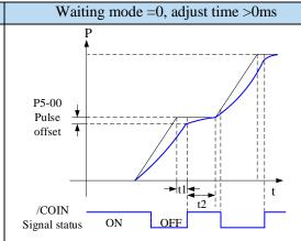
After the drive output 1-segment position command, it will wait for the completion of motor positioning, and pass the adjust time, then start the next position command. T1 is positioning time, t2 is adjust time. Refer to parameter P4-11.
