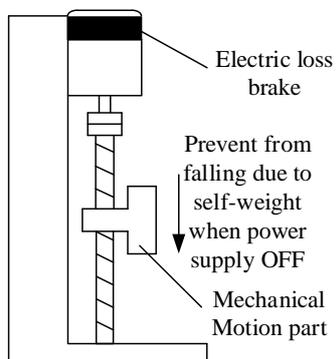
Note: The brake built in the servo motor is a fixed special brake without excitation. It can not be used for dynamic braking. Please use it only when the servo motor is in a stop state.
