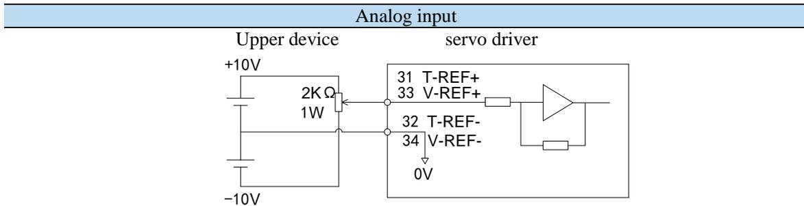
Note: Analog Pin31 (External Torque Analog Differential Input+), 32 (External Torque Analog Differential Input-), 33 (External Speed Analog Differential Input+), 34 (External Speed Analog Differential Input-) are soldered out of the CN0 port as detailed in chapter 3.1.3.1.
