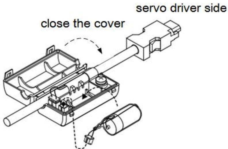
(5) After replacing the battery, in order to remove the "Encoder Battery Alarm (E-222)" display, please do clear alarm twice (F0-00=1).
