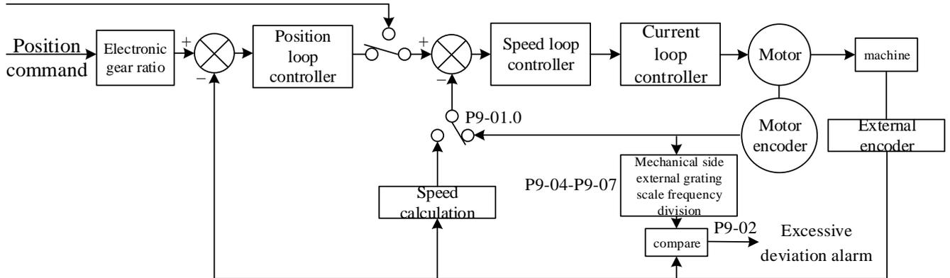
When the full closed-loop is opened, the external grating ruler position feedback is used; when the full closed-loop speed feedback is opened, the external grating ruler speed feedback is used. When the full closed-loop mode is on, the control mode can be switched (P0-01 and P0-02).
