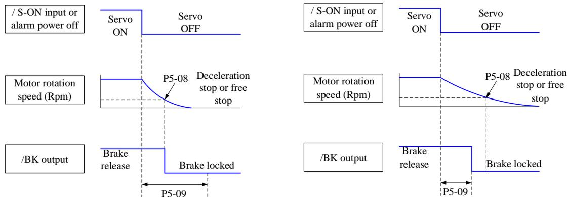
Since the brake of the servo motor is designed to be used as a position holder, it must be activated at the right time when the motor stops. While observing the action of the machine, adjust the user's parameters.
