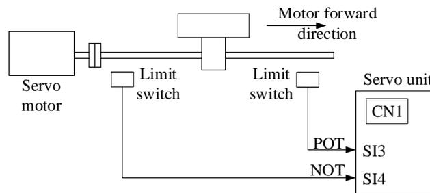
Rotary applications such as round tables and conveyors do not need the function of overrun prevention. At this time, there is no need to connect the overrun prevention with input signals.
