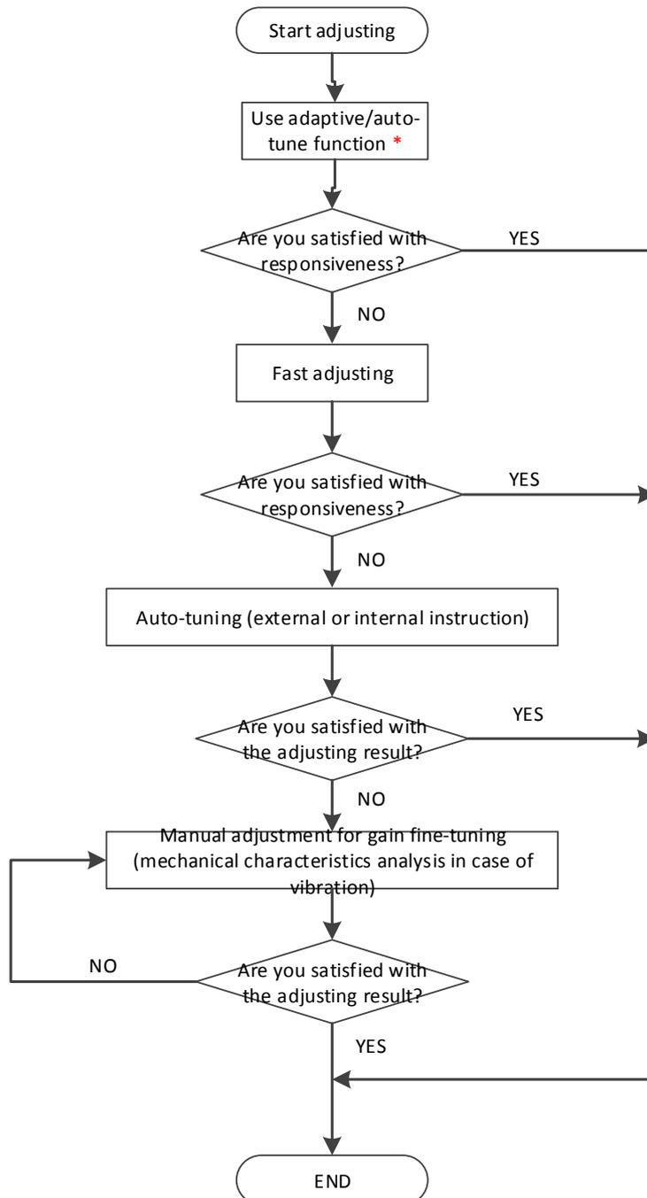
Note: \* 3KW and below models use auto-tune mode (hardware version before 3730 is adaptive mode), above 3KW models use adaptive mode.
