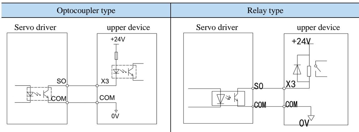
Note: The maximum load current is 400 mA (if the brake motor is controlled by SO<sub>x</sub>, please confirm the brake current first, and if it is larger than 400 mA, please use the intermediate relay).
