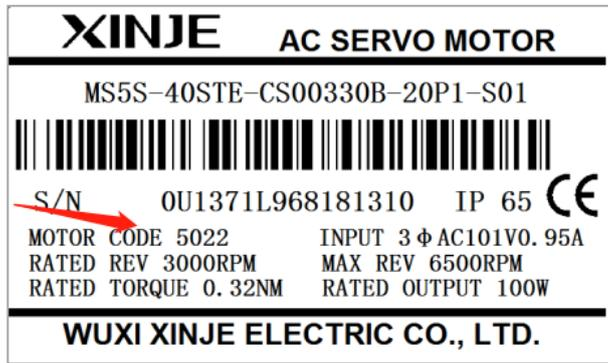
Note: Errors in motor code setting will prompt E-310 (motor code error), which can be set again after F0-00 clears the alarm.
