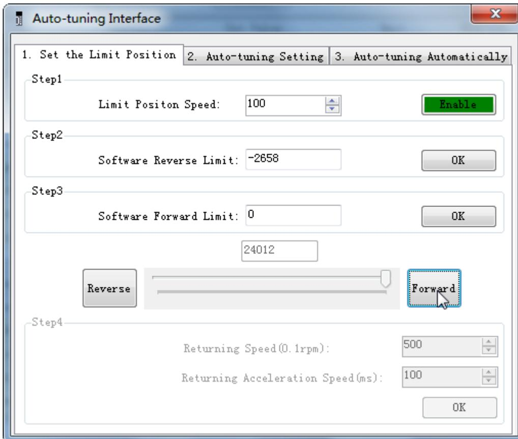
2. Select jog or manual setting to configure the trip of inertia identification.
