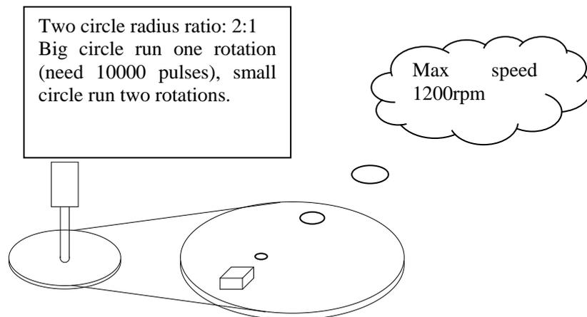
Set the actual length per command pulse for precise positioning. For example: the object moves 1um per command pulse. The command pulses of load rotating one circle = 6mm / 1um = 6000. In the case of deceleration ratio is 1:1, set pulse per rotation P0-11=6000, P0-12=0. Then if the PLC outputs 6000 pulses, the object will move 6mm.
