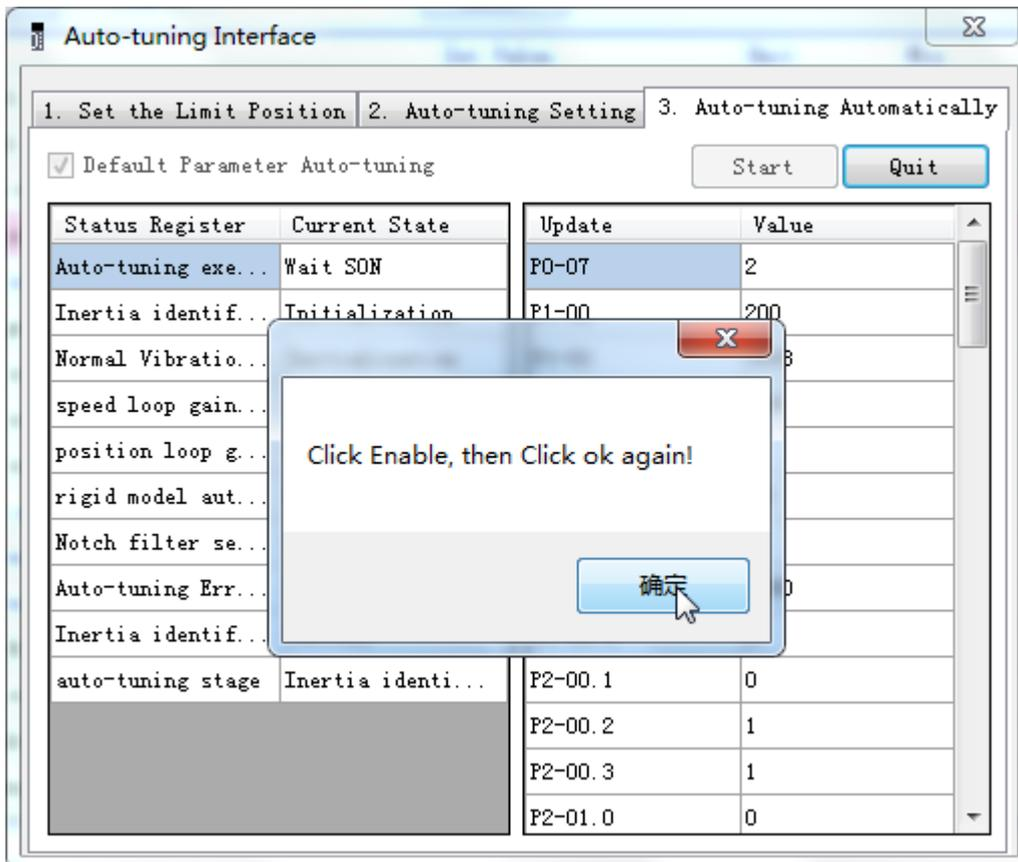
8. The upper device starts to send pulses, wait the completion of auto-tuning.
