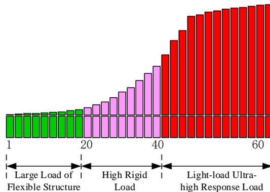
Flexible structure large load: refers to the type of synchronous belt structure, large load inertia equipment.
