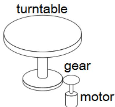
Because it can only rotate in one direction, after a certain period of time, the number of revolving cycles will always exceed the upper limit of absolute value encoder.
