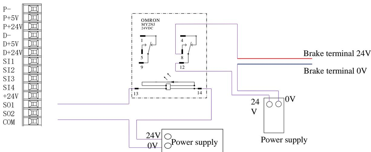
1. P5-44 defines the terminal of the brake output signal. As shown in the figure above, the S01 controls brake, that is, P5-44 = 0001.
