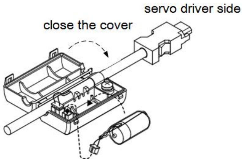
(5) After replacing the battery, in order to remove the "Encoder Battery Alarm (E-222)" display, please restore the factory settings and cut off the power supply of the servo unit;
