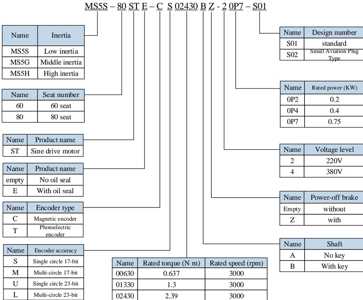
Note: At present, only the combination of CS, CM, TL and T is selected for the type of encoder.
