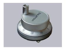
The output signal of the hand pulse generator must be OC (collector open circuit signal) DC24V type. Generally, there will be five wires, three signal wires (A, B, Z), two power wires (24V, 0V), signal wires connected with the corresponding high-speed counting input port of the PLC. The power supply can be supplied by the output 24V of the PLC or by the switching power supply.
