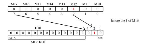
If the number of bits in the source address is 1, the high bit side is ignored, and if the source address is 0, the instruction will not be executed.
