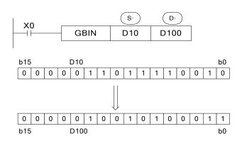
From the left second bit of D10, XOR each bit with the value after decoding, as the bit value after decoding (the left bit will not change). The transformation value will be stored in D100.
