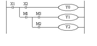
LD X1 MCS LD X2 OUT Y0LD M1MCS LD M3 OUT Y1 LD M2 OUT Y2 MCR MCR
