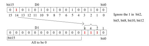
If the number of bits in the source address is 1, the low side is ignored, and if the source address is 0, the instruction will not be executed.
