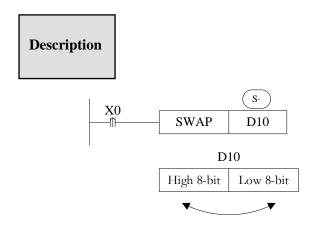
Exchange the high 8-bit and low 8-bit of 16-bit register.
