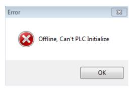
In both cases, use PLC system update tool to update PLC system, and PLC and PC will be connected successfully if system is updated (For more steps about system update, please refer to Q3 related content).
