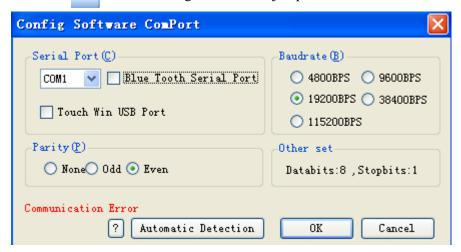
Choose correct communication serial port according to your PC actual serial port.; baud rate selects 19200BPS, parity check selects even parity, 8 data bits, 1 stop bit; you can also click 'check' button directly in the window, and communication parameters will be selected by PLC itself. 'Connect PLC successfully' will be displayed on the left bottom of window as below:
