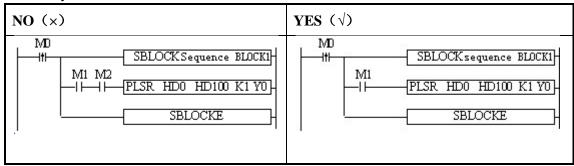
The SKIP condition only can use M, X, can not use other coil or register.
