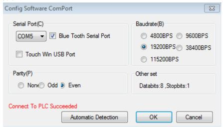
Then it means that PLC has been connected to PC successfully!
