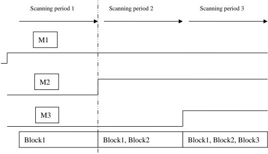
Note: When the program in the BLOCK is not executed and the triggering condition M is disconnected, the BLOCK will not stop immediately, but will complete the last scan, and will stop after the rest of the program has been executed.
