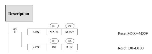
$\bigcirc$  D1)  $\bigcirc$  Are specified as the same type of soft units, and  $\bigcirc$  D1) <  $\bigcirc$  D2)
