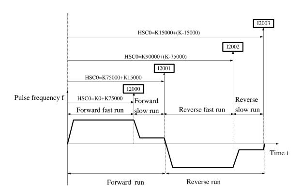
Below is PLC program: Y2 represents forward output signal; Y3 represents reverse output signal; Y4 represents output signal of speed 1; HSC2: Back-forth times accumulation counter; HSC0: AB phase HSC;
