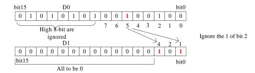
If multiple bits in the source address is 1, the low side is ignored, and if the source address is 0, the instruction will not be executed.
