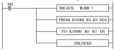
Note: As shown in the figure above, in V3.4 and above version software, when the module number is set to K0~K15, the corresponding ladder diagram will be displayed as K10000~K10015.
