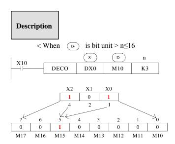
N=3, so the decoding object is the lower three bits in DX0, which are  $X2 \sim X0$ .
