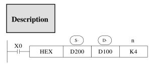
Convert the high 8 bits and low 8 bits in source  $\bigcirc$  to HEX data. Move 4 bits every time to destination  $\bigcirc$  . The convert character number is assigned by n.
