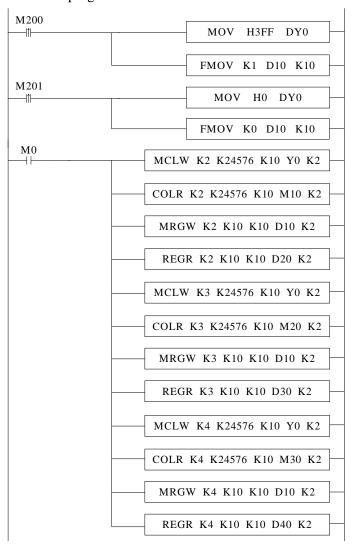
//at the rising edge of M200, set ON the master PLC Y0~Y11, D10~D19 are set to 1, at the rising edge of M201, set OFF Y0~Y11 of master PLC, reset D10~D19.
