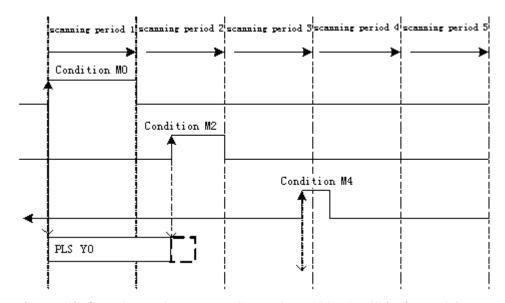
When M0 is from OFF→ON, run "PLSR HD0 HD100 K1 Y0" in the BLOCK to output the pulse;
