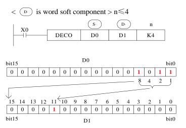
The low n-bit (n  $\leq$ 4) of the source address is decoded to the target address. When n  $\leq$  3, the high 8-bit of the target turns to 0.
