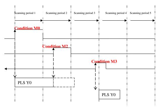
When M0 is OFF→ON, run 'PLSR HD0 HD100 K1 Y0' in the BLOCK to output the pulse; When M2 is OFF→ON, the BLOCK stops running, the pulse output stops at once; When M3 is OFF→ON, output the rest pulses.
