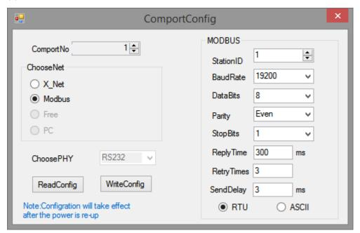
Serial port: K0 ~ K5. Port0 (RS232), Port1 (RS232), Port2 (RS485) or Port2-RS232 (RS232) or Port2-RS485 (RS485), Port3 (left extension port), Port4 (upper extension port 1), Port5 (upper extension port 2).
