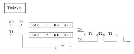
X0 is ON, Y0 begin to twinkle. T1 is Y0-OFF time; T2 is Y0-ON time.
