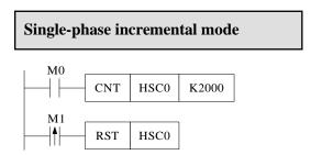
When the M0 is ON, HSC0 counts the rising edge of the OFF to ON of the input X0 port at high speed.
