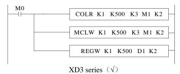
Note: XD/XL series PLC sequence block has cancelled Modbus communication instructions, which is replaced by the current Modbus instruction handling mode.
