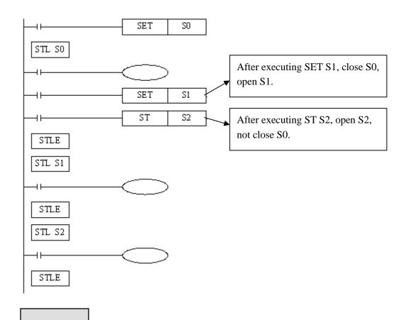
Example 1: the flows run in branch then merge in one flow. Program diagram:
