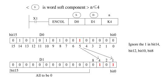
If multiple bits in the source address is 1, the high bit side is ignored, and if the source address is 0, the instruction will not be executed.
