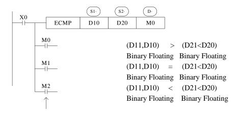
When X0 is OFF, even ECMP doesn't run, M0~M2 will keep the status before X0 is OFF.
