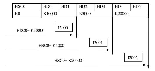
Note: When absolute counting is performed in non-cam mode, counting interrupts are generated sequentially, i.e., segment 1 interruption, segment 2 interruption, segment 3 interruption... When a segment interrupt occurs, no interrupt occurs even if the count value reaches the set value of the segment again.
