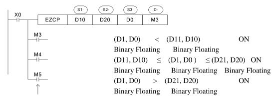
When X0 is OFF, even EZCP doesn't run, M3~M5 will keep the status before X0 is OFF.
