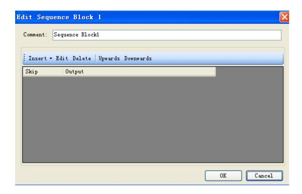
You can edit the BLOCK in the window, Upwards/Downwards are used to change the position of instructions in the block.
