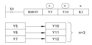
As the following picture, when the data address overlapped, the instruction will do from 1 to 3.
