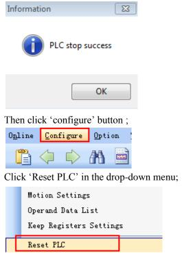
By this time, 'Reset PLC' information window will jump out and it means that all steps of 'Stop when PLC reboot' have been finished.
