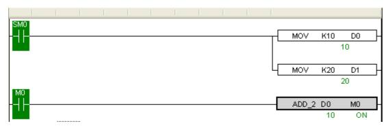
(5) From Free Monitor in the toolbar, we can see that D2 changes to be 30, it means assignment is successful;
