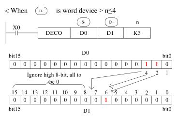
The low n-bit (n  $\leq$  4) of the source address is decoded to the target address. When n  $\leq$  3, the high 8-bit of the target turns to 0.
