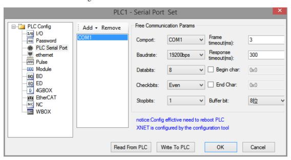
**Port No.**: It refers to Port of PLC, COM0 refers to Port 0 (RS232), COM1 refers to Port 1 (RS232), COM2 refers to Port 2 (RS485) or Port 2-RS232 (RS485) or Port 2-RS485 (RS485), COM3 refers to Port 3 (left extended ED port), COM4 refers to Port 4 (upper extended BD port 1), COM5 refers to Port 5 (upper extended BD port 2).
