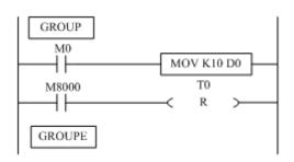
Generally, GROUP and GROUPE instruction can be programmed according to the group's function. Meantime, the programmed instructions can be FOLDED or UNFOLDED. To a redundant project, these two instructions are quite useful.
