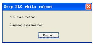
By this time, cut off PLC power for 2-3s and power on again, then a 'PLC has been stopped successfully' window will normally jump out; if the window do not jump out after power on, try again a few times until the information window of successful stop jump out.
