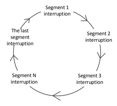
Via setting SFD331, users can switch between single loop mode or continuous loop mode. The detailed assignment is show below:
