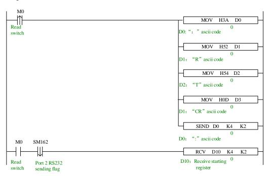
When trying to communicate between PLC and other intelligent devices, it is suggested to use serial debugging tool to determine the data format of communication, that is, protocol. The advantages of this method are: the serial debugging tool is easy to modify and flexible to use; after the serial debugging tool determines that communication can be successful, the PLC
