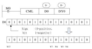
Each data bit in the source device is reversed  $(1 \rightarrow 0, 0 \rightarrow 1)$  and sent to the destination device. If use constant K in the source device, it can be auto convert to be binary. This instruction is fit for PLC logical converse output.
