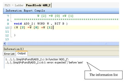
According to the information shown in the output blank, we can search and modify the grammar error in C language program. Here we can see that in the program there is no ';' sign behind W [2] = W[0] + W[1].
