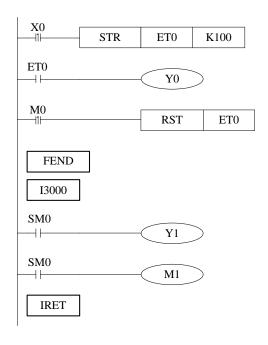
When X0 changes from OFF to ON, ET0 will start timing. And ET0 reset when accumulation time is up to 100ms; meantime generates an interruption, the program jumps to interruption tag I3000 and execute the subprogram.
