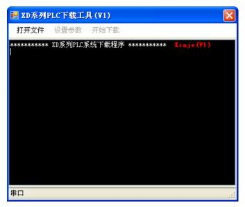
Click "Open File", choose the PLC model for updating. (Note: XD3\_16.sys fit for PLC model XD3-16, XD3\_60.sys fit for PLC model XD3-32 and XD3-60):
