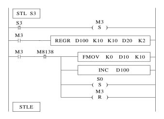
//read the D10~D19 of slave PLC 2, 3, 4 to master PLC D20~D29, reset D10~D19 after the communication is successful, then the station no. is added 1, process S0 is executed, cycle.
