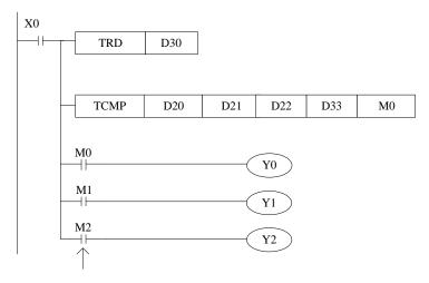
The present clock is 15:32:49 7,30,2014 Wednesday. So D30=14, D31=7, D32=30, D33=15, D34=32, D35=49, D36=3. If the setting time is 15:32:49, D20=15, D21=32, D22=49, so Y1=ON. If the setting time is 17:32:49, D20=17, D21=32, D22=49, so Y0=ON. If the setting time is 2:32:5, D20=2, D21=32, D22=5, so Y2=ON.
