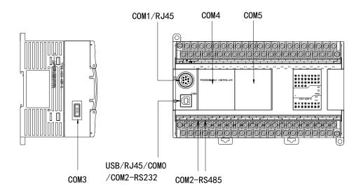
Note: The left side of output terminal block of XD5E/XDME/XDH is RS232 port.
