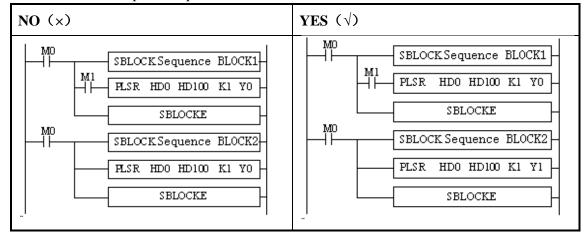
Do not use the same pulse output terminal in BLOCK and main program.
