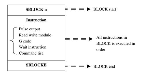
$\times$ 1: Firmware version below V3.4.5: the XD series PLC allows up to eight BLOCKs. Firmware version V3.4.5 and above: XD/XL series PLC can write up to 100 BLOCKs, but at the same time can only run 8.
