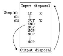
PLC repeatedly carries on input disposal, program executing and output disposal. If write END instruction at the end of the program, then the instructions behind END instruction won't be executed. If there's no END instruction in the program, the PLC executes the end step and then repeats executing the program from step 0.
