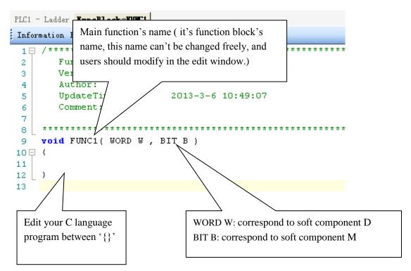
• Parameters' transfer way: if call the **Function Block** in ladder, the transferred D (HD) and M (HM) is the start ID of W and B. Take the above graph as the example, start with D0 and M0, then W[0] is D0, W[10] is D10, B[0] is M0, B[10] is M10; if the parameters in the ladder are HD0, HM0, then W[0]=HD0,B[0]=HM0; if the parameters in the ladder are D100, HM100, then W[0]=D100, B[0]=HM100. So, word and bit components start address are defined in PLC program by the user.
