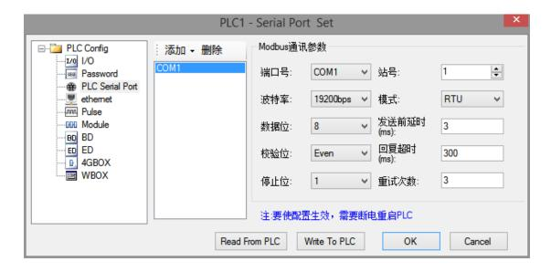
**Port No.**: It refers to Port of PLC, COM0 refers to Port 0 (RS232), COM1 refers to Port 1 (RS232), COM2 refers to Port 2 (RS485) or Port 2-RS232 (RS485) or Port 2-RS485 (RS485), COM3 refers to Port 3 (left extended ED port), COM4 refers to Port 4 (upper extended BD port 1), COM5 refers to Port 5 (upper extended BD port 2).
