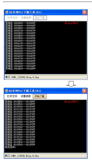
After finishing the update, cut off the PLC power, take off the short jumper, then power on the PLC again.
